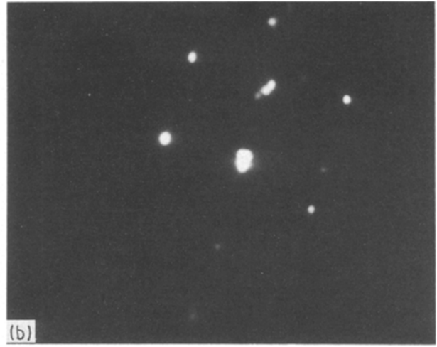
Figure 9 Transmission electron micrograph of a particle near a damaged fibre in the weld. (a) Bright-field image. (b) Electron diffraction pattern taken from (a). (c) Key diagram of diffraction pattern.
